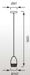
SILA Pendant 1. MD1510-1 (white) 2. MD1510-1 (chrome) 1*G9 MAX 42W white or chrome glass / metal chrome IP20
